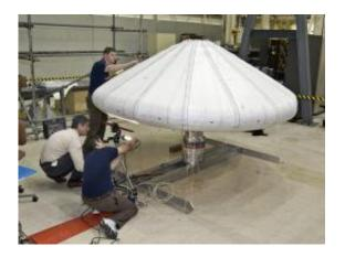
NASA engineers check out the Inflatable Re-entry Vehicle Experiment (IRVE) in the lab. Credit: NASA/Sean Smith
