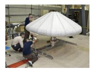
NASA engineers check out the Inflatable Re-entry Vehicle Experiment (IRVE) in the lab. Credit: NASA/Sean Smith
