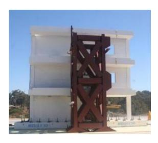
Engineers tested the seismic response of a 1920s-era masonry building at the UC San Diego Englekirk Structural Engineering Center.
