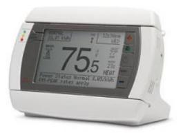
Berkeley engineers are working on a smart home thermostat that could save energy costs and resources by using settings to crank the air conditioning down at night or when occupants are out. First-generation devices, which appeared during the 1970s oil crisis, are often not programmed because owners find them too confusing. PHOTO COURTESY THE RESEARCHERS
