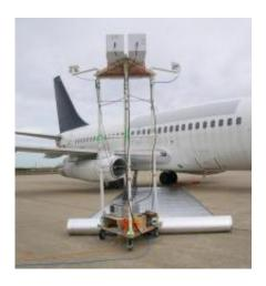
This photo shows testing equipment being used by NIST scientists in recent research mapping radio frequency penetration of airframes, in this case a Boeing 737-200. The data from the tests provided valuable independent data on how electromagnetic radiation penetrates commercial aircraft, thereby helping improve safety. Credit: NIST
