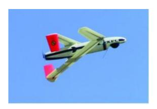
NRL and its fuel cell development and manufacturing partner, Protonex Technology Corporation (Southborough, MA) have addressed these issues by developing a hydrogen <u>fuel cell</u> power plant system that greatly extends endurance and permits increased payload capacity. The technology has been successfully integrated into the XFC UAS, a folding wing, expendable UAS that has a small footprint with a standard lightweight rail launcher.
