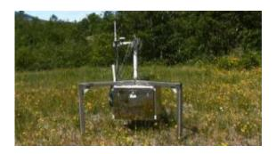
A sensor like this is being placed inside and around the mouth of Mount St. Helens. One day it may be used to respond rapidly to an impending eruption.
