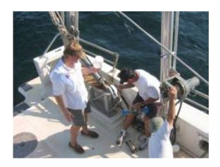
Estes (center), Al-Hamdan (right), and a Mississippi State graduate student (left) check water samples. The instrument in the picture is lowered into the water and samples trapped at various depths.
