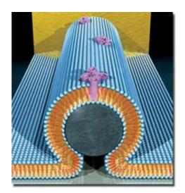
An artist's representation of a nanobioelectronic device incorporating alamethycin biological pore. In the core of the device is a silicon nanowire (grey), covered with a lipid bilayer (blue). The bilayer incorporates bundles of alamethicin molecules (purple) that form pore channels in the membrane. Transport of protons though these pore channels changes the current through the nanowire. Image by Scott Dougherty, LLNL
