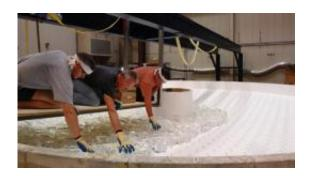
Casting team members at the Steward Observatory Mirror Lab loading 22,500 pounds of E6 Ohara borosilicate glass into the 6.5-meter honeycomb mold for the San Pedro Mártir Telescope mirror. (Ray Bertram, Steward Observatory, University of Arizona)
