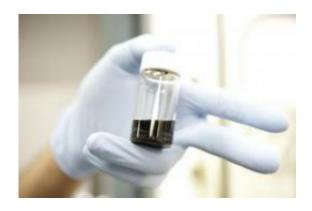
At the core of Korgel's research are the nanoparticle "inks" (as shown here) which are the sunlight-absorbing materials of his solar cells. Credit: Beverly Barrett, UT Engineering Public Affairs
