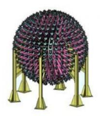
General Fusion's reactor design consists of 220 pistons that simultaneously ram a metal sphere. This creates a shock wave inside the sphere, so that plasma rings in the center create a fusion reaction. Credit: General Fusion.
