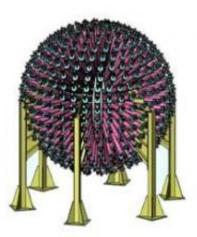
General Fusion's reactor design consists of 220 pistons that simultaneously ram a metal sphere. This creates a shock wave inside the sphere, so that plasma rings in the center create a fusion reaction. Credit: General Fusion.
