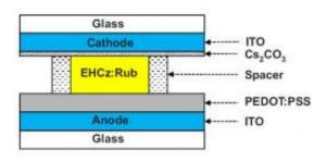
The new liquid-OLED has a liquid semiconducting layer made of EHCz doped with rubrene. Liquid-OLEDs could offer improved device reliability and greater flexibility. Credit: Xu and Adachi.
