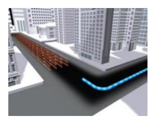
A single superconducting cable (shown in blue) could one day replace a dozen traditional copper cables (shown in red), freeing up much needed space beneath city streets. Credit: DHS S&T
