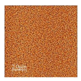
Gold surfaces created by other methods are substantially rougher, and would result in many of the molecular switches either being smashed or not contacting the silicon. Credit: Coll Bau, NIST
