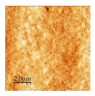
The flip-chip lamination method creates an ultra-smooth gold surface, which allows the organic molecules to form a thin yet even layer between the gold and silicon. Credit: Coll Bau, NIST
