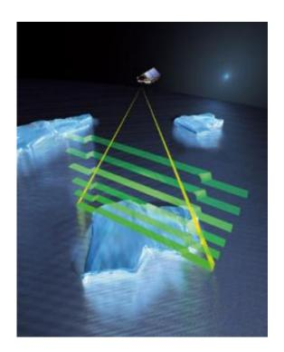
Using a sophisticated radar altimeter called SIRAL (Synthetic Aperture Radar Interferometric Radar Altimetry), CryoSat-2 will make accurate measurements of the thickness of floating sea-ice so that seasonal to inter-annual variations can be detected. It will also survey the surface of continental ice sheets to detect small elevation changes. Credits: ESA - AOES Medialab
