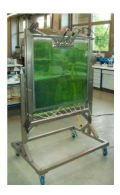
This is a newly developed plate reactor for an optimum light management in the
