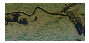
Airborne radar image of the Tropisar test site. The colour composite illustrates the information content of radar images. Dark areas correspond to water bodies, for example the river in the centre of the image, and marsh areas below the river. The green areas represent forests with image tone reflecting different forest characteristics. Credits: ONERA
