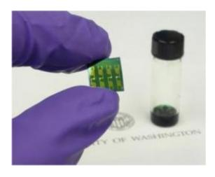
An organic polymer circuit that transports both positive and negative charges. The circuit was created by solution casting of a newly developed material. Credit: University of Washington
