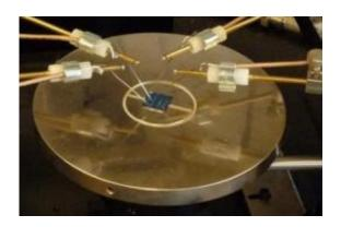
The organic circuit developed at the University of Washington that transmits positive and negative charges. Here it is undergoing a test. Credit: University of Washington
