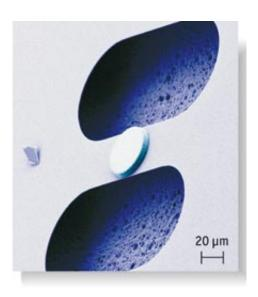
A small round mirror (middle) is attached to a mechanical bridge such that photons hitting the mirror are reflected and exert a force onto it. Photo: IQOQI
