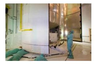
On Launch Pad 39A, technicians check the clearance of the payload bay door as it closes around the multi-purpose logistics module Leonardo and the lightweight multi-purpose experiment support structure carrier inside space shuttle Discovery's payload bay. Photo credit: NASA/Jack Pfaller
