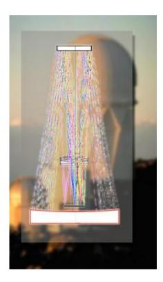
The Mayall 4-meter telescope at Kitt Peak National Observatory can be adjusted to observe a 3-degree field of view with a high-precision spectrograph. A new secondary mirror (top) and a corrector and field flattener will send the light to a flat focal plane (above primary mirror) where the light from each target object is carried to spectrographs by optical fibers.
