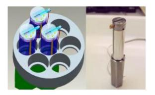
Robot actuators individually position each optical fiber precisely where it needs to be to collect the light from a specific astronomical object programmed by
