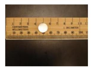
An efficient catalyst is needed to get the half liter of hydrogen out of this small, 240 mg pellet of solid ammonia borane. Credit: Pacific Northwest National Laboratory
