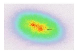
A high-resolution absorption image of a heterogeneous sample of Mottinsulating, superfluid and normal gases of ultracold atoms in an optical lattice. Each pixel corresponds to a square 660nm on a side, and the optical resolution is 1.3 micron. Credit: Cheng Chin, James Franck Institute, University of Chicago
