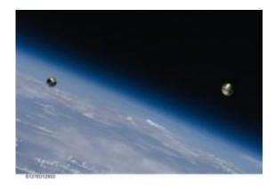
The ANDE-2 spacecraft, Castor and Pollux, shortly after deployment from Space Shuttle Endeavour on July 30, 2009, as photographed by the crew of STS-127 from the flight deck. Credit: NASA
