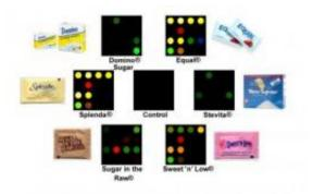
In an advance toward a long-awaited "electronic tongue," a new sensor can detect up to 14 commonly-used sweeteners. The device shows promise for quality control monitoring in the food and beverage industry. Credit: Kenneth Suslick, Ph.D., University of Illinois at Urbana-Champaign
