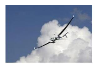
The Antares DLR-H2 flies its madden voyage over the northern German city of Hamburg. The airplane powered by fuel cells was commissioned by the German Aerospace Centre (DLR) with the goal of developing fuel cells for a reliable onboard power supply for wide-body airliners.
