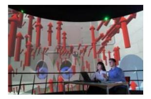
Engineers developing a combustion plant use a new VR model to study the direction in which gases will flow through it. Credit: Dirk Mahler / Fraunhofer IFF
