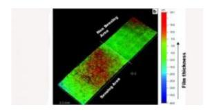
This is topography of inkjet-sprayed PVAm, and AChE (50 U/mL) and DTNB doped sodium silicate (SS) thin films on paper. Credit: McMaster University
