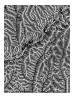
Overhead view of Gabilan Mesa, California, showing the logarithm of drainage area, calculated by routing flow computationally over an elevation map from the National Center for Airborne Laser Mapping (NCALM). Light shades are ridgelines, darker shades are valleys. Scene is approximately 3.5 km wide. Courtesy / Taylor Perron (MIT)
