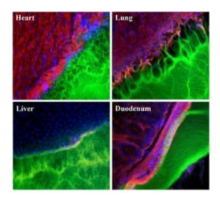
Images showing the interface between a surgical glue (green) and tissue samples (red, blue and black) from the heart, lung, liver, and duodenum. The glue works best with duodenum tissue (note smooth interface), and worst with lung tissue (pockmarked with holes). Courtesy / Edelman lab/MIT
