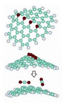
Princeton engineers will study how fuel additives made of tiny particles of graphene can help supersonic jets fly faster and make diesel engines cleaner and more efficient. To create the graphene particles, the researchers remove carbon dioxide molecules from graphite oxide (top two molecules) which leaves a irregular bond pattern that creates a buckle in the otherwise flat graphene molecule (bottom molecule). This ridge prevents the graphene molecule from folding into ball.
