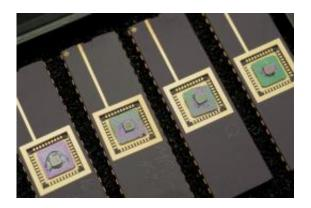
Ohio State University researchers have coated these microsensor silicon chip arrays, which were provided by collaborators at the National Institute of Standards and Technology, with tiny particles of nickel oxide. Once further developed, this technology could lead to sensors that detect toxic industrial chemicals and biological warfare agents. Photo by Jo McCulty, courtesy of Ohio State University.
