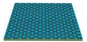
Graphene consists of carbon atoms only one atomic layer thick, with the unique characteristic that its electrons behave as if they have zero mass. Credit: Lau lab, UC Riverside.
