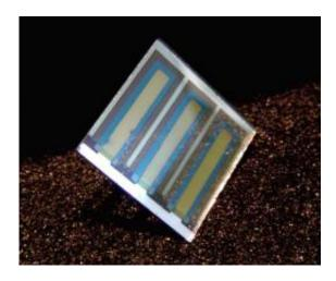
An organic photovoltaic cell on glass. The goal for UA scientists is to understand and control the interfaces in these devices at nanometer-length scales (less than 1/100,000 the thickness of a human hair) to enable the development of long-lived solar energy conversion devices on tough, flexible and extremely low-cost plastic substrates.
