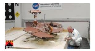
Rover driver Paolo Bellutta measures how much the rover moved sideways, downslope, during the maneuver.
