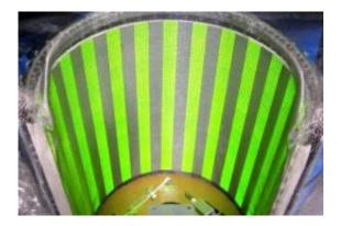
Moving pictures displayed here simulate flight for an immobilized fly; electrodes give researchers a window into the fly's neural activity and vision processing.
