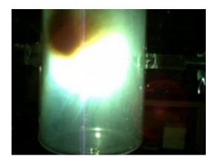
Lead rods, which are infused with the material to be encapsulated in hollow carbon molecules known as fullerenes, are blasted with a plasma arc. The resulting soot contains the filled carbon molecules. The remote-control process was invented to insert radio-labeled materials into fullerenes for use in diagnosing and treating tumors. Brain tumors are the target of the NIH-funded research being carried out by a Virginia Tech-Virginia Commonwealth University team. Credit: Harry Dorn
