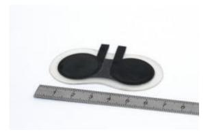
The small, thin battery comes out of the printer and can be applied to flexible substrates. Credit: Fraunhofer ENAS
