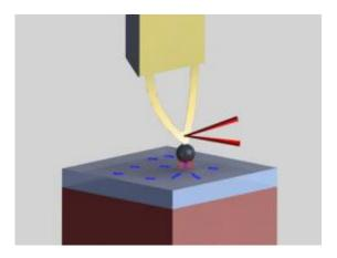
A diagram of the setup, including a cantilever from an atomic force microscope, used to measure the heat transfer between objects separated by nanoscale distances. Courtesy / Sheng Shen
