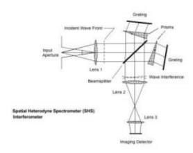
This is a schematic diagram of the Spatial Heterodyne Hpectrometer (SHS) Interferometer. Credit: Naval Research Laboratory
