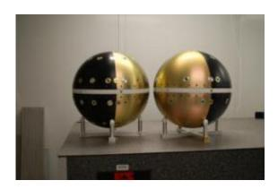
ANDE-2 consists of two spherical microsatellites, Pollux and Castor, that are both 19" in diameter but have different masses. ANDE-2 is a low-cost mission designed to study the atmosphere of the Earth from low-Earth orbit by monitoring total atmospheric density between 300 and 400 km altitude. Credit: NRL photo
