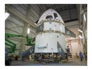
The Max Launch Abort System (MLAS) test vehicle features fixed fins and drag plates to inexpensively, yet effectively, simulate deployable fins or other aerodynamic devices that would be used on an operational launch vehicle. Credit: NASA/Sean Smith
