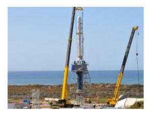
On Launch Complex 576-E at Vandenberg Air Force Base in California, NASA's Orbiting Carbon Observatory, OCO, upper stack is lowered toward the Stage 0 motor of the Taurus XL vehicle. Image credit: NASA/Randy Beaudoin
