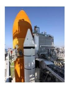
In this image provided by NASA the afternoon sun creates shadows on space shuttle Endeavour's external fuel tank as workers remove the seal from the Ground Umbilical Carrier Plate on the tank Wednesday June 24, 2009. A hydrogen leak at the location during tanking for the STS-127 mission caused the launch attempts to be scrubbed on June 13 and June 17. NASA plans a fueling test Wednesday July 1, 2009 of shuttle ahead of July 11 launch attempt. (AP Photo/NASA)
