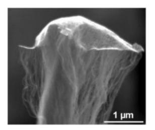
An odako grown at Rice University shows single-walled nanotubes lifting an iron and aluminum oxide "kite" as they grow while remaining firmly rooted in a carbon base.
