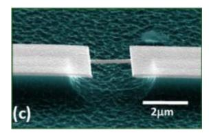
This photo shows scanning electron micrographs showing one of the doublyclamped beam NEMS devices used in these experiments. It is embedded in a nanofabricated three-terminal UHF bridge circuit. Credit: Fabricated by Akshay Naik and Selim Hanay in the Roukes lab and the Kavli Nanoscience Institute/Caltech.
