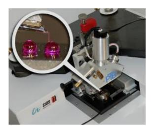
The micro probe used in the micro-nano CMM measures the form and the spacing of two reference spheres with diameters of two millimetres each. The figure shows a survey of the system and the proportions of measuring probe and measurement object in detail. (Image: PTB)
