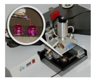
The micro probe used in the micro-nano CMM measures the form and the spacing of two reference spheres with diameters of two millimetres each. The figure shows a survey of the system and the proportions of measuring probe and measurement object in detail. (Image: PTB)
