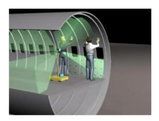
ONR's laser image projection technology eliminates reliance upon traditional paper templates and string measurements and equips production workers with direct access to CAD model information needed to locate/mark points of attachment for electrical and ventilation hangers, studs, piping, sound damping and other fixed point attachments. Credit: Office of Naval Research
