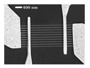
Scanning electron microscope image shows ten graphene nanoribbons between each pair of electrodes.
