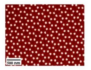
(PhysOrg.com) -- The first artificial graphene has been created at the NEST laboratory of the Italian Institute for the Physics of Matter (INFM-CNR) in Pisa. It is sculpted on the surface of a gallium-arsenide semiconductor, to which it grants the extraordinary properties of the original graphene. Published as a Rapid Communication on *Phys.Rev.B*, the research has been highlighted by the American Physical Society.
